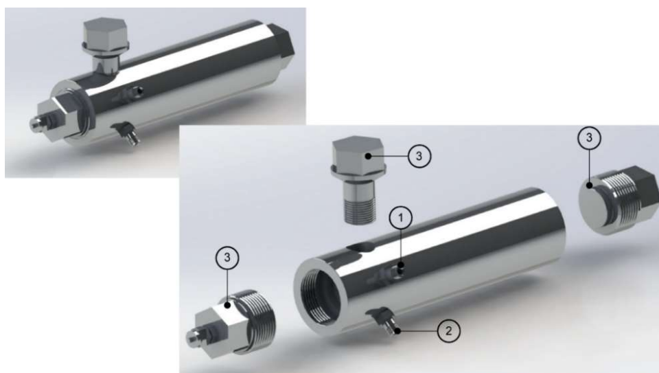
Figure 3.4. Equilibrium cell in high-pressure configuration. (1) Pressure and charging connections; (2) temperature measurement; (3) blind plugs.
