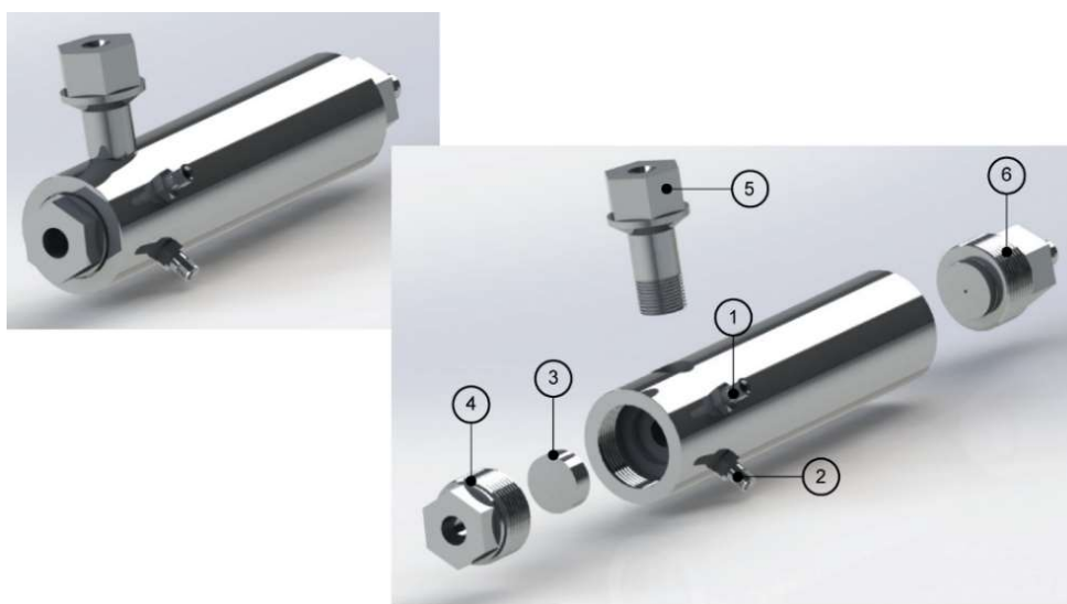
Figure 3.3 Equilibrium cell in visualization configuration. (1) Pressure and charging connections, (2) temperature measurement, (3) sapphire window, (4) front plug, (5) illumination window and (6) back plug.
