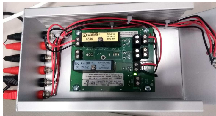
Figure 19 – Amplifier box built with 8B40 module
