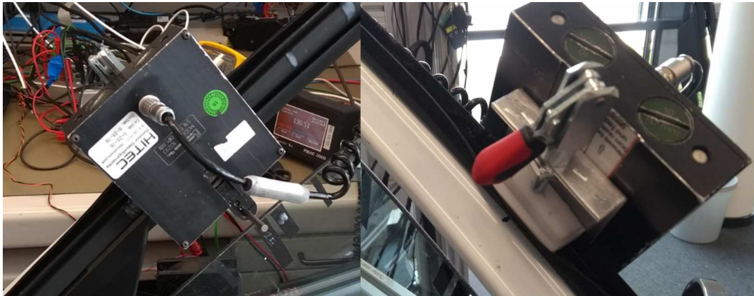
Figure 29 – SDI fixed on the door frame
