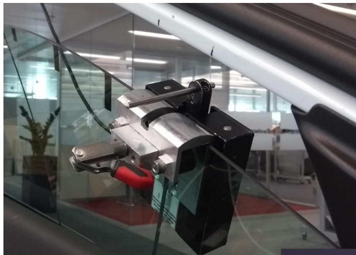
Figure 15 – SDI force gauge fixed on the window
