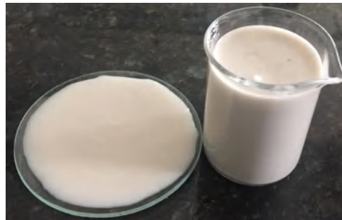
Figure 4.1 – Water-based drilling fluid with xanthan gum and limestone.
