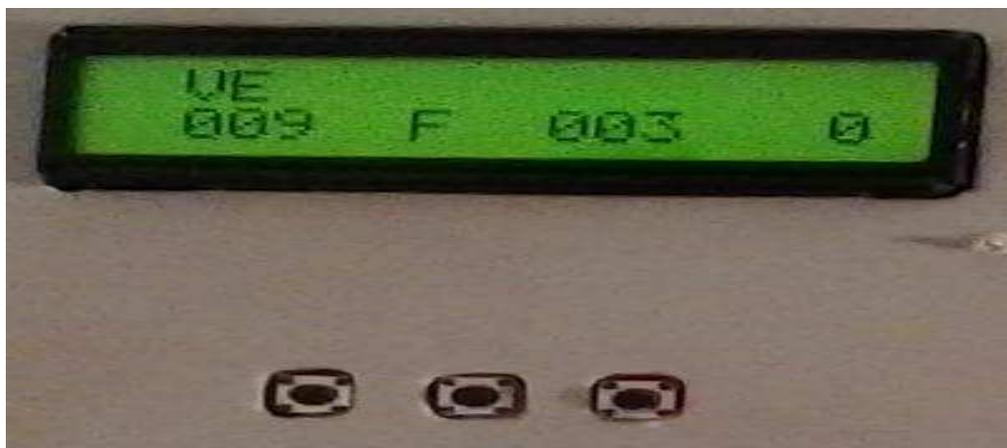
**Figura 17: – display LCD 16 X 2**
