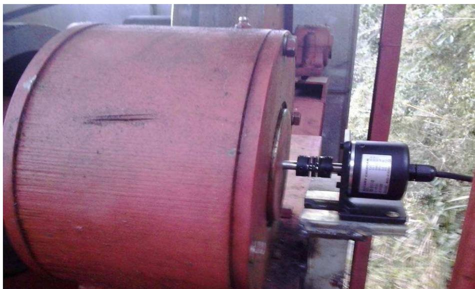
**Figura 15: – encoder incremental instalado**
