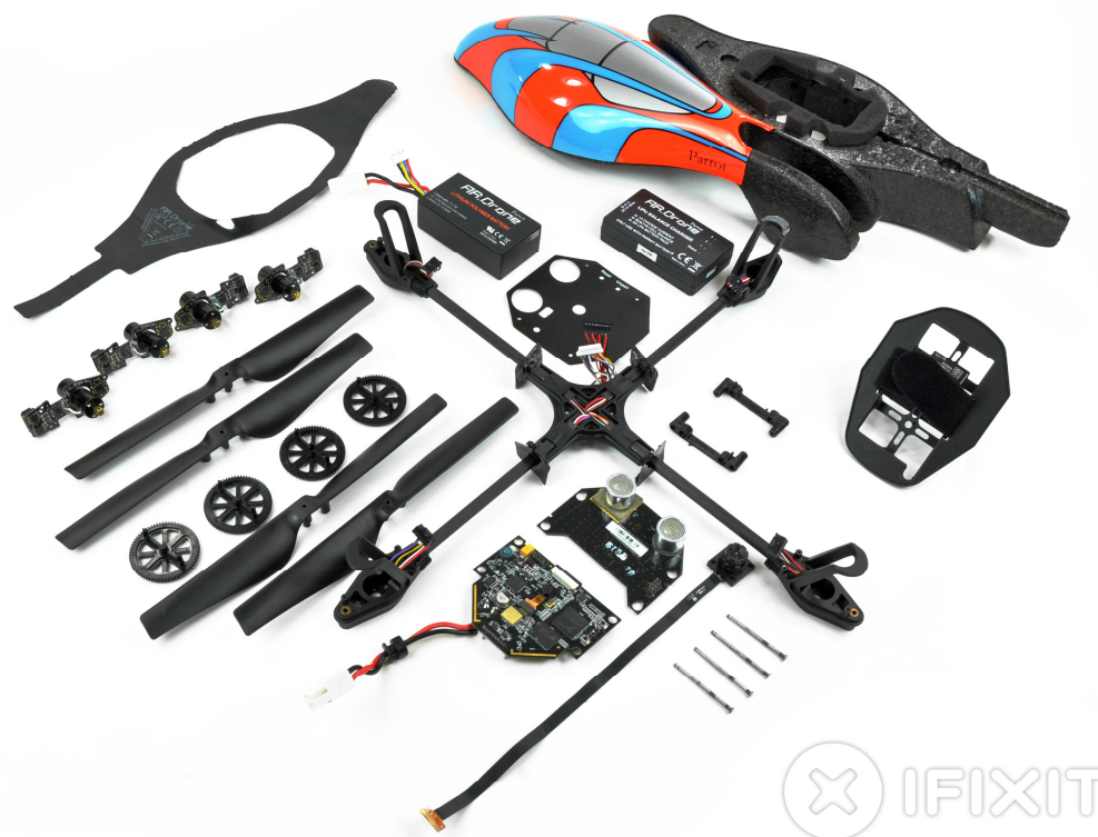
Figura 4 – Componentes do ArDrone 2.0. Fonte: https://www.ifixit.com/Device/Parrot_AR.Drone .
