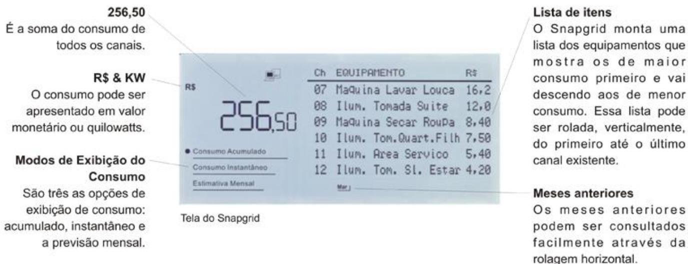
Figura 6 - Interface do SnapGrid.
