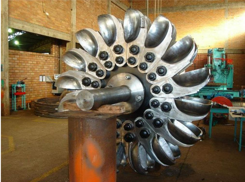
Figura 13 – Turbina Pelton
