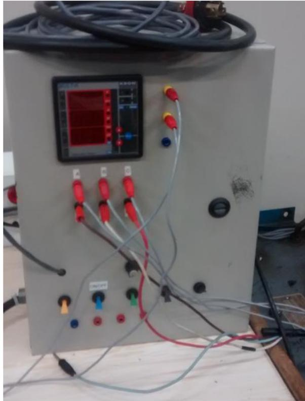
**Figura 25 – Multimetro Mult-K.**
