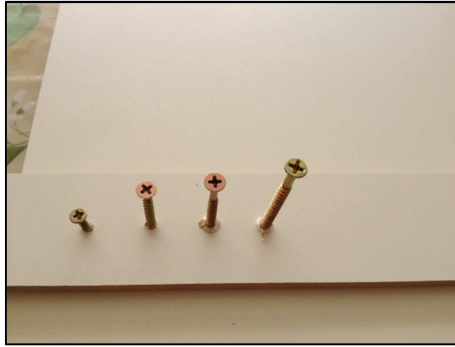
Figura 91: Parafusos (mini 200 mm C x 6 mm \varnothing ); (pequeno 300 mm C x 6 mm \varnothing ); (médio 400 mm C x 6 mm \varnothing ) e (grande 500 mm C x 6 mm \varnothing ).
