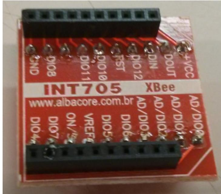
FIGURA 26 – SOQUETE XBEE
