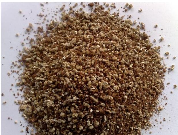
Figura 2.8 – Vermiculita expandida
