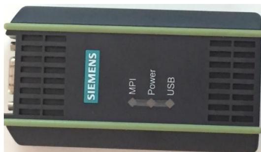
Figura 13 - Conversor Siemens USB – MPI.
