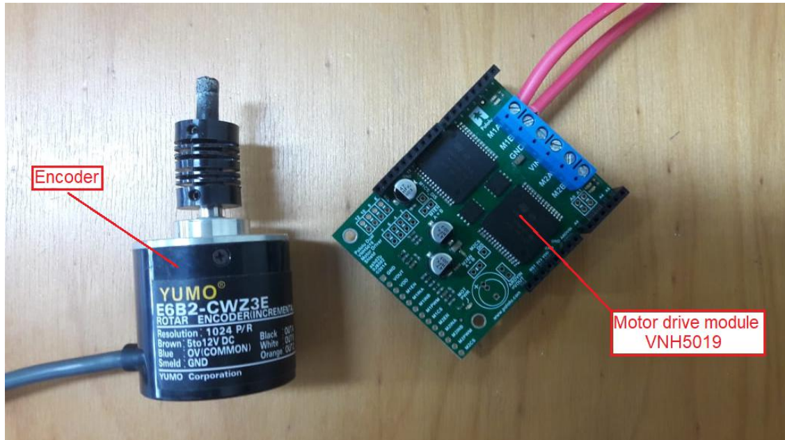
Photograph 1 – Encoder and DC motor drive module
