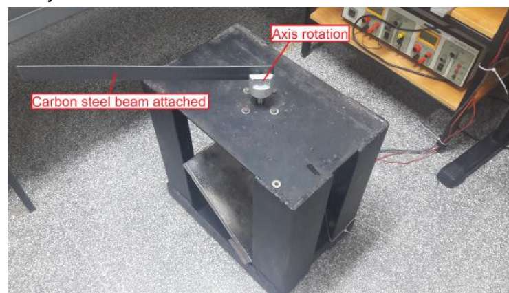
Photograph 4 – DC motor system
