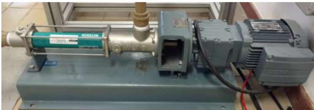
Figura 3.4 - Bomba helicoidal NEMO NM 021BY.
