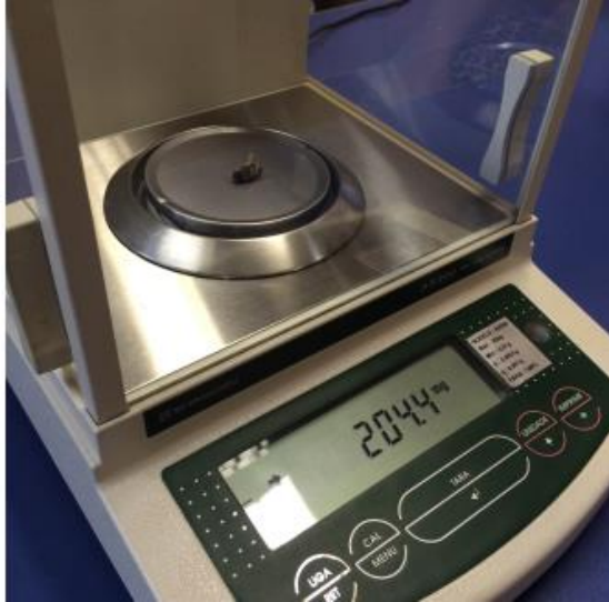
Picture 3: Precision scale balance (0.0001g) Shimadzu/AX 200
