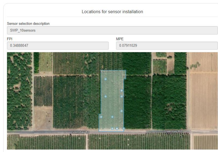
Figure 35 – Locations determined for sensor installation using 10 sensors and SWP sample.
