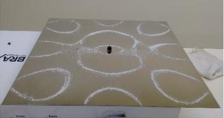
A photograph of a square Chladni plate with a central black dot. The plate is covered with a fine layer of white sand. At 758 Hz, the sand has formed a pattern of several concentric, roughly circular curves. The word "BRAX" is visible on the left side of the plate.                                            |
