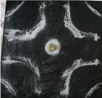
A Chladni plate pattern at 565 Hz, showing a central yellow circular spot surrounded by a single white ring, with four white curved lines extending from the corners towards the center, forming a more complex, star-like shape.                            |
