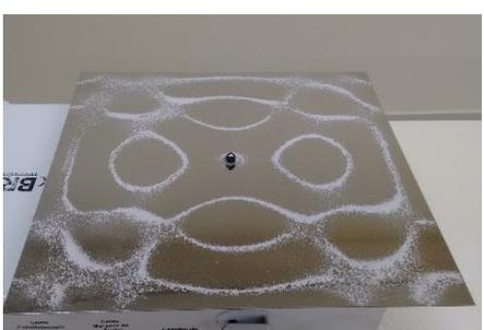
A photograph of a square Chladni plate with a central circular hole. The plate is covered with a layer of fine white sand. At a frequency of 1.213 Hz, the sand has formed a pattern of four large, rounded lobes arranged in a cross shape, with smaller lobes at the corners. The plate is mounted on a wooden base with various control knobs and switches visible at the bottom. |
