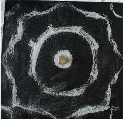
A Chladni plate pattern at 904 Hz, showing a central yellow circular spot surrounded by a single white ring, with four white curved lines extending from the corners towards the center, forming a more complex, star-like shape.                            |
