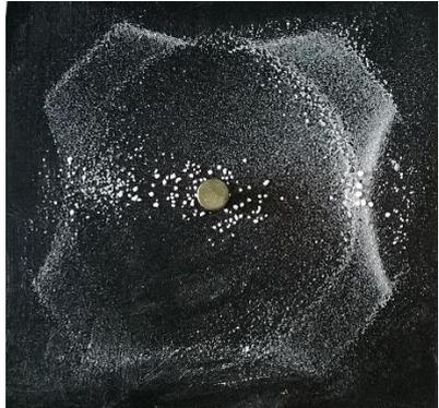
A Chladni plate experiment showing a central yellow circular object surrounded by a dense, irregular ring of white sand particles. The ring is roughly square-shaped and represents the third overtone mode.                                              |
