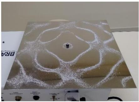
A photograph of a square Chladni plate with a central circular hole. The plate is covered with a layer of fine white sand. At a frequency of 1.000 Hz, the sand has formed a pattern of four large, rounded lobes arranged in a cross shape, with smaller lobes at the corners. The plate is mounted on a wooden base with various control knobs and switches visible at the bottom.   |
