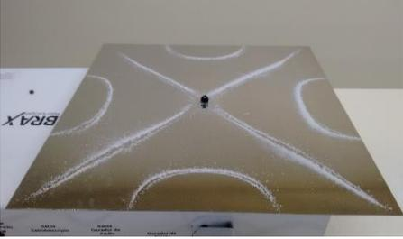
A photograph of a square Chladni plate with a central black dot. The plate is covered with a fine layer of white sand. At 386 Hz, the sand has formed a pattern of four curved lines that meet at the center, creating a cross-like shape with rounded ends. The word "BRAX" is visible on the left side of the plate. |
