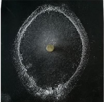
A Chladni plate experiment showing a central yellow circular object surrounded by a dense ring of white sand particles. The ring is roughly circular and represents the second overtone mode.                                                             |
