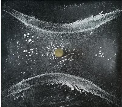
A Chladni plate experiment showing a central yellow circular object surrounded by a sparse distribution of white sand particles. Two distinct, curved lines of sand are visible, one above and one below the center, representing the first overtone mode. |
