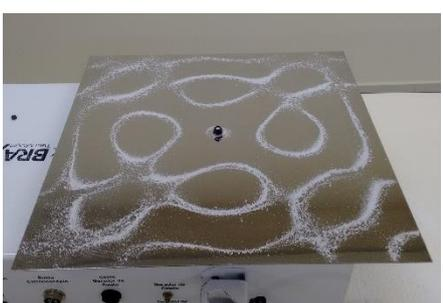
A photograph of a square Chladni plate with a central circular hole. The plate is covered with a layer of fine white sand. At a frequency of 1.209 Hz, the sand has formed a pattern of four large, rounded lobes arranged in a cross shape, with smaller lobes at the corners. The plate is mounted on a wooden base with various control knobs and switches visible at the bottom.   |
