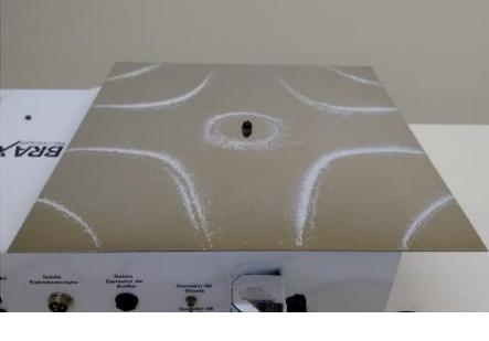
A square Chladni plate with a central pivot point. The sand has formed a pattern of curved lines that create a central circular region surrounded by several curved, parallel lines, resembling a stylized flower or a complex lattice. |
