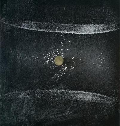
A Chladni plate experiment showing a central yellow circular object surrounded by a sparse distribution of white sand particles. Two distinct, curved lines of sand are visible, one above and one below the center, representing the first overtone mode.  |
