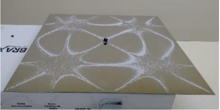
A photograph of a square Chladni plate with a central black dot. The plate is covered with a fine layer of white sand. At 786 Hz, the sand has formed a complex pattern of interconnected, irregular curves that resemble a web or a lattice structure. The word "BRAX" is visible on the left side of the plate.    |
