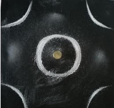
A Chladni plate pattern at 209 Hz, showing a central yellow circular spot surrounded by a single white ring, with four white curved lines extending from the corners towards the center.                                                                       |
