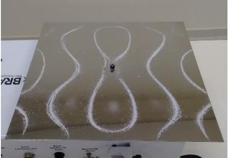
A photograph of a square Chladni plate with a central black dot. The plate is covered with a fine layer of white sand. At 690 Hz, the sand has formed a pattern of two vertical, teardrop-shaped curves that meet at the center. The word "BRAX" is visible on the left side of the plate.                             |
