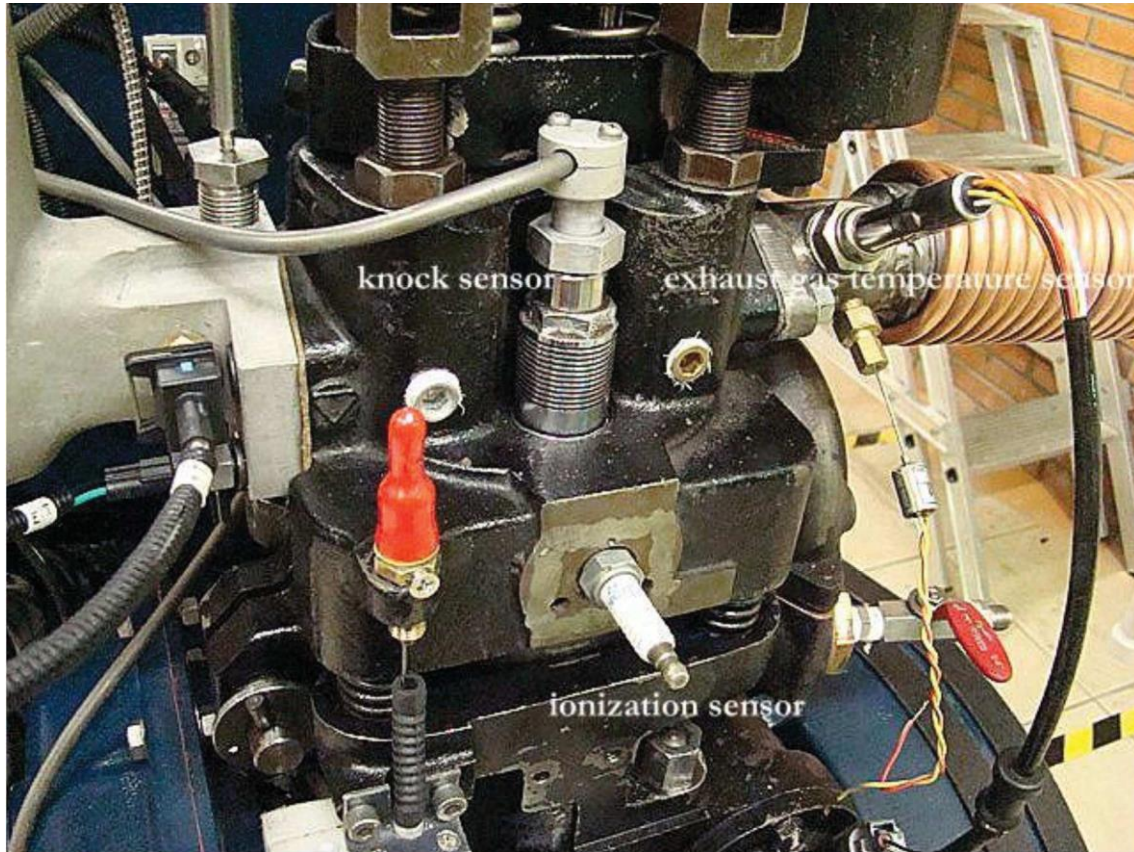
Figure 2: Modified CFR engine, showing the ionization sensor position.
