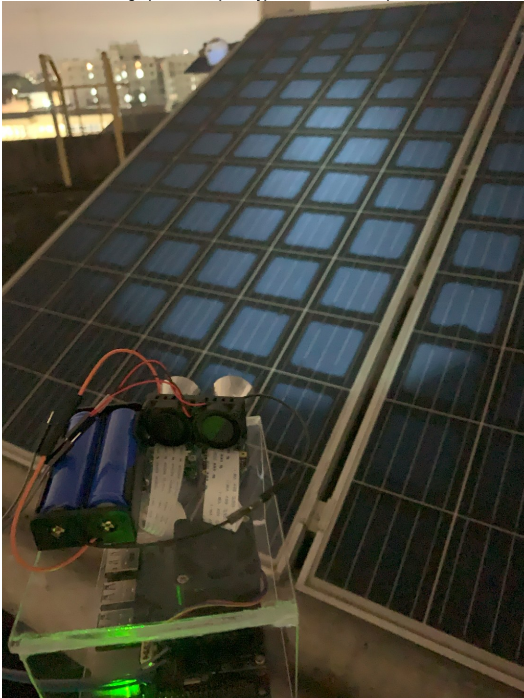
Photograph 4 - First prototype used for UVF inspection.
