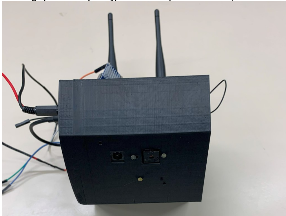
Photograph 8 - Third prototype with the 3D printed involucre, front vision.
