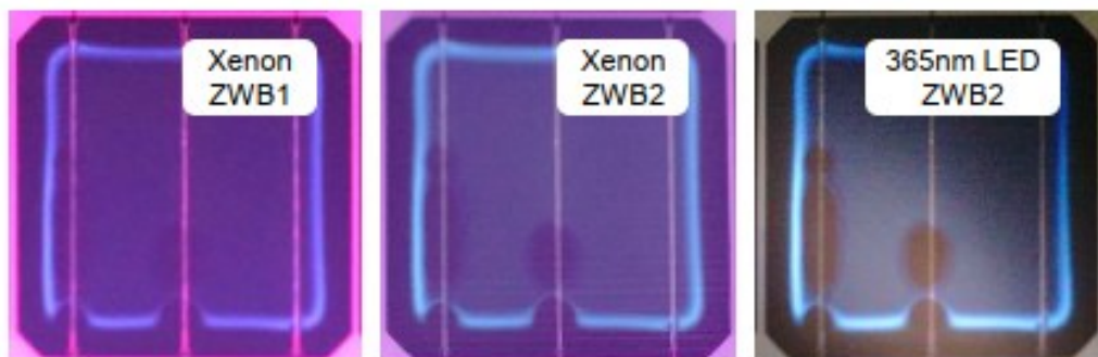
Figure 12 - Same cell with three different types of UV illumination. Xenon flash with ZWB1 filter on the left, xenon flash with ZWB2 filter in the middle and 365 nm LED flashlight with ZWB2 filter in the right.
