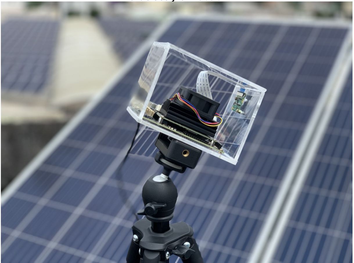
Photograph 3 - First prototype version with the Jetson Nano, Raspberry Pi Camera Module 2 and the acrylic involucre.
