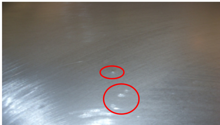
Figure 4 – Samples of imprint defects (highlighted by red circles). Source: Author.
