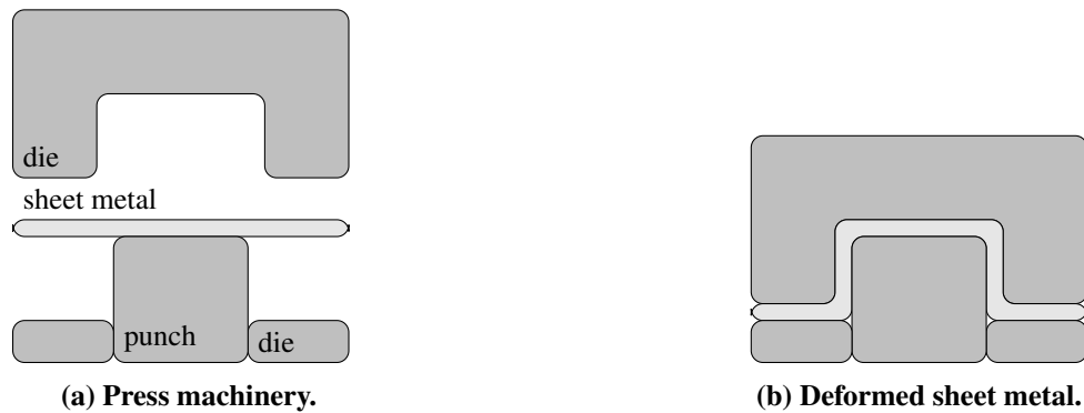
Figure 2 – Stamping machinery: a punching force deforms a sheet metal using a modeling die. Source: Author.
