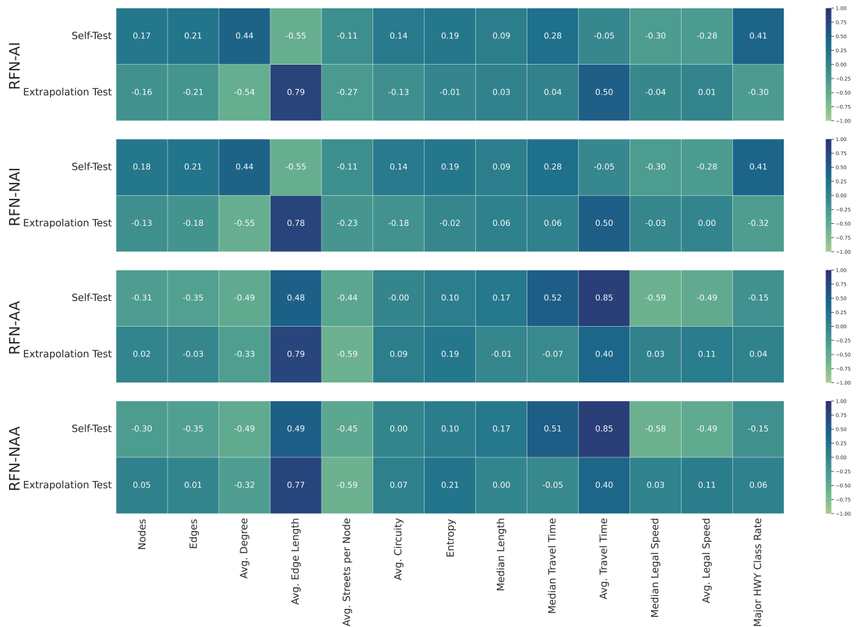
Figure 30 – Heatmap of Pearson correlations between a road network feature (column label) and the corresponding regression error of cities for self-test and extrapolation-test in each RFN variant (row label).
