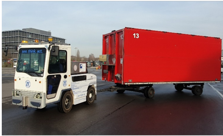
Figure 7 – Electric ZF's VOLK Tugger : the vehicle is coupled with a red trailer which has a 2-axle turntable steering.
