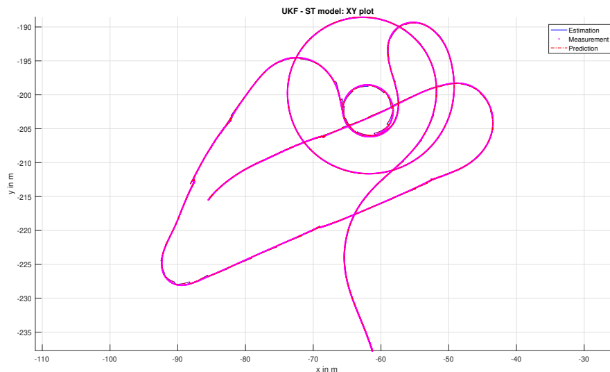
Figure 57 – Estimation of the trajectory of the vehicle test using the UKF: this figure shows the plot for the estimates, the measurements and the predictions of the filter. The estimations are equal to the predicted results when the GNSS values are not available.
