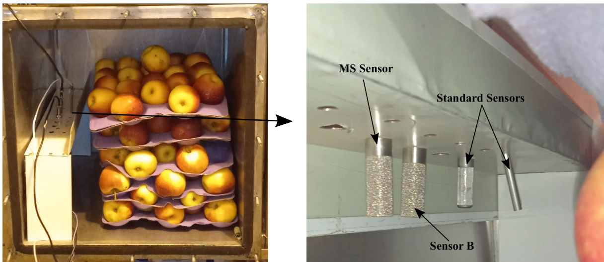
Figure 7 – Setup of the sensor verification. On the right is a photo of the test chamber, installed in a cold chamber. On the left is a detail of the sensor installation.
