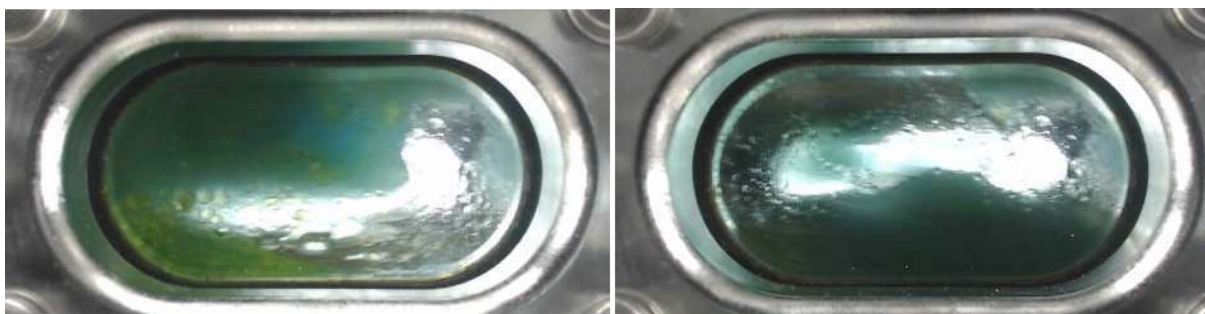
Figure 5.17— Photo from experiment #70 (80 %vol. LL, 70 %vol. WC, 18.75 rpm) showing the detachment of the upper hydrate deposit: the imminence of the sloughing event (left) and right after it has occurred (right).
