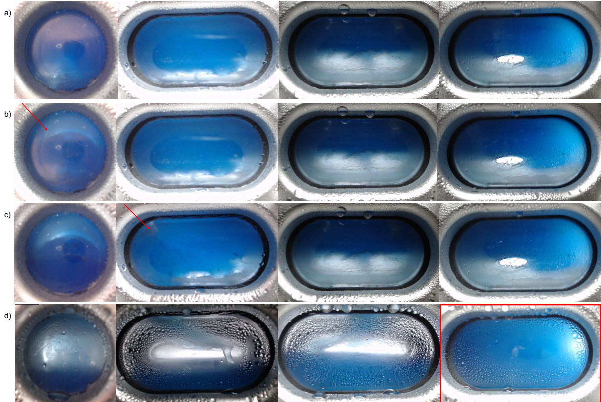
Figure 4.11— Photos from the experiment #10 (50 %vol. LL and 18.75 rpm) showing the rock-flow cell before the sloughing events (a), two consecutive sloughing events (b, c) with time between shots of 2 and 26 seconds after the beginning of the hydrate formation. The red arrow shows the window where the rupture of the hydrate deposit occurred. The red rectangle highlights the window where the plug formation occurred.
