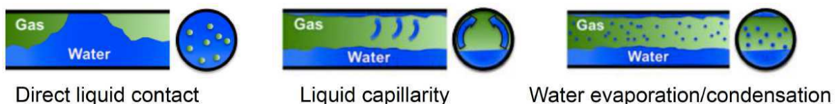
Figure 2.6 – Mechanisms of water migration to the deposition surface.
