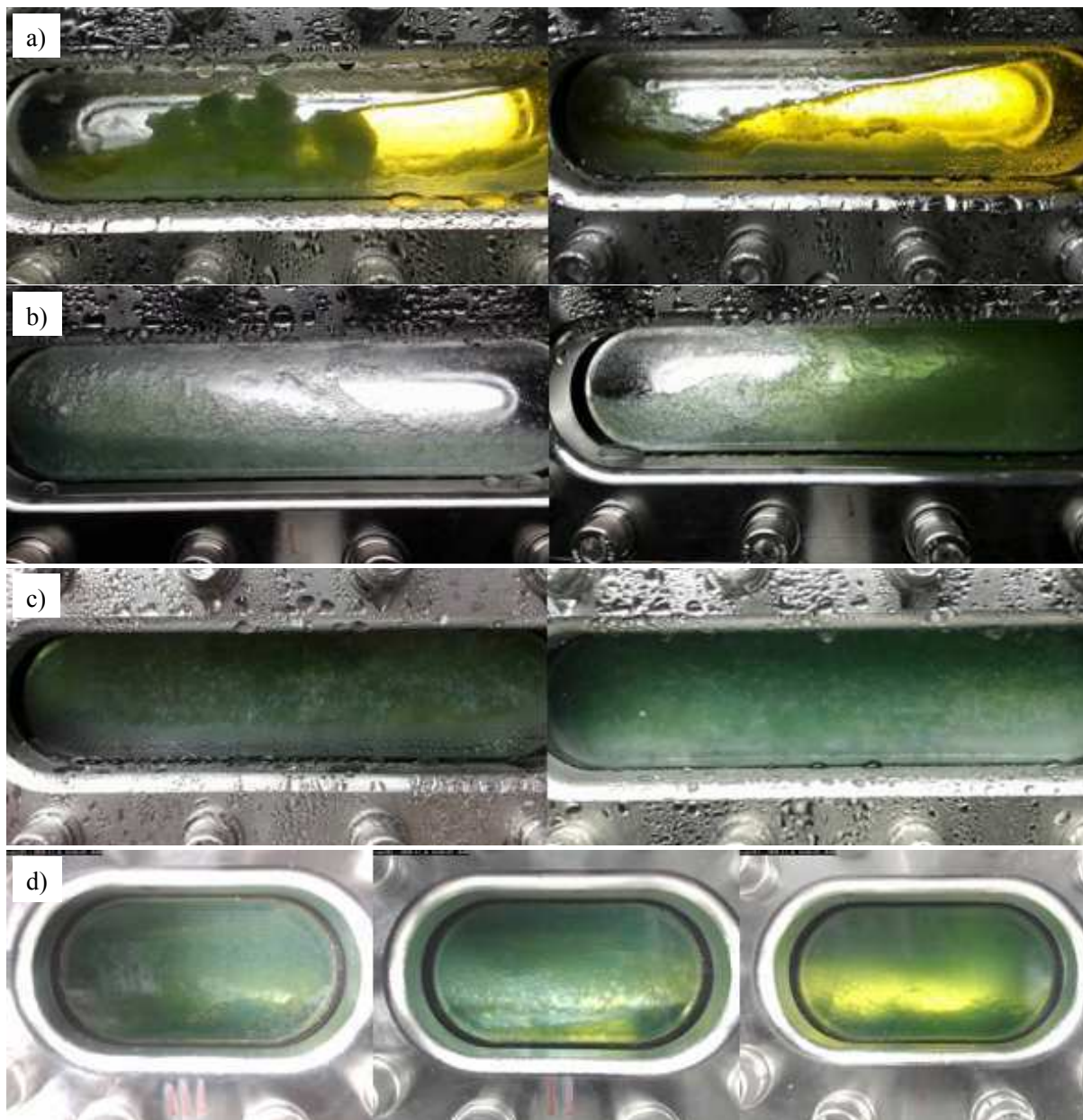
Figure 5.13— Captured images of the rock-flow cell: a) experiment #57 (60 %vol. LL, 20 %vol. WC and 11.25 rpm) representing the conditions for low water content and low to medium liquid loading system, b) experiment #47 (40 %vol. LL, 45 %vol. WC and 11.25 rpm) representing the conditions for middle water content (20 to 45 %vol.) and for low to medium liquid loading (40 to 60 %vol. LL), c) experiment #58 (60 %vol. LL, 70 %vol. WC and 18.75 rpm) representing the conditions for high water content (> 45%vol.) and low to middle liquid loading (40 to 60 %vol. LL), d) experiment #69 (80 %vol. LL, 70 %vol. WC and 11.25 rpm) representing the conditions for high liquid loading (> 60 %vol. LL).
