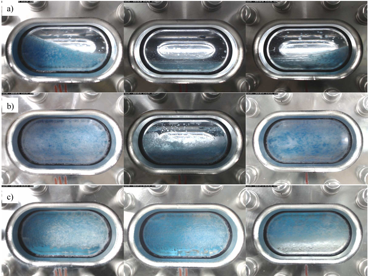
Figure 4.5— Captured images of the rock-flow cell experiments taken 48 hours after the beginning of the hydrate formation showing the final hydrate morphology: a) experiment #20 (20 %vol. LL and 06 rpm) presents a bottom wall deposit, b) experiment #25 (40 %vol. LL and 11.25 rpm) shows a plug formation at the edges of the rock-flow cell, c) experiment #39 (60 %vol. LL and 06 rpm) show a thicker upper wall deposit with some unconverted water at the bottom.
