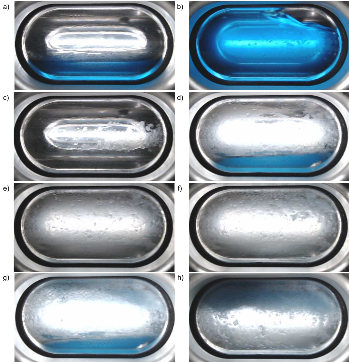
Figure 4.7— Images captured before the onset of the hydrate formation a) of experiment #28 (40 %vol. LL and 06 rpm), at the beginning of the hydrate formation b), hydrates adhered to the wall c), after the first wave due to the oscillation of the rock-flow cell d), second wave e), third wave f), 140 and 200 seconds after the beginning of the hydrate formation g) and h), respectively.
