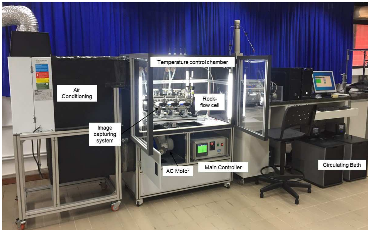
Figure 3.2— Rock-flow cell system with six front viewing windows.
