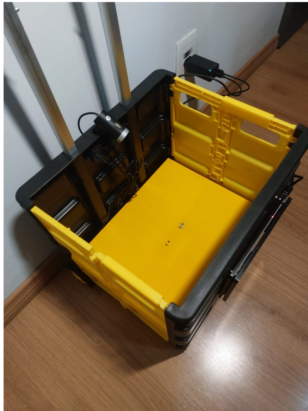
Figure 44 – Top view of the assembly showing the false bottom
