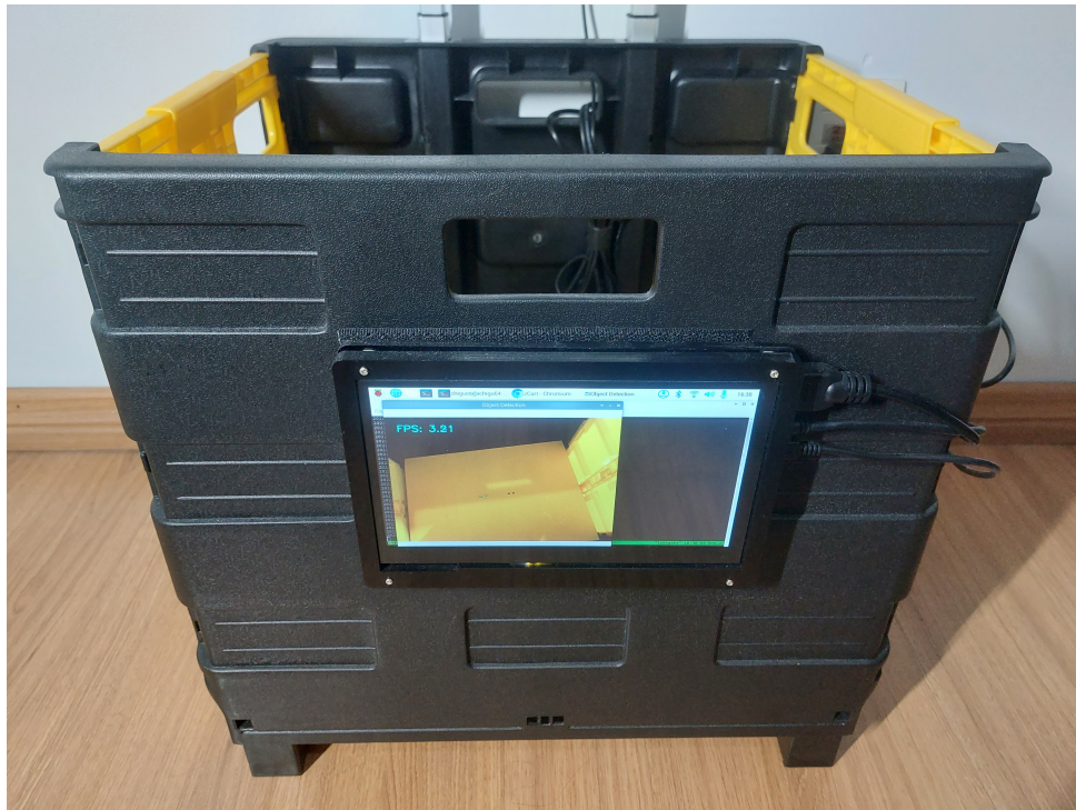
Figure 62 – Frontal view of the prototype displaying the video camera feed
