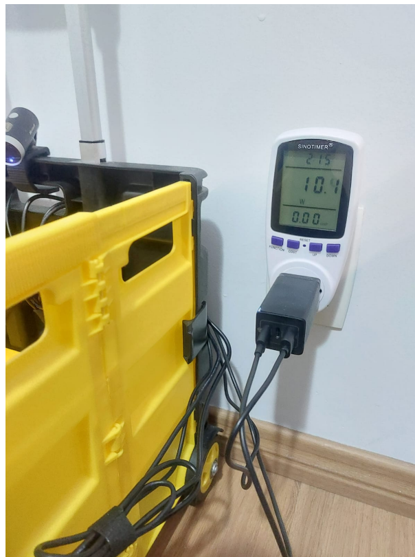
Figure 54 – Power consumption measurement using a wattmeter
