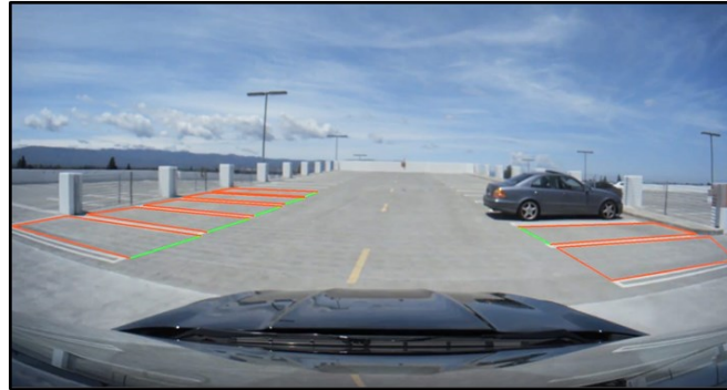
Photograph 4 - ParkNet, a deep neural network developed to detect parking spaces using images
