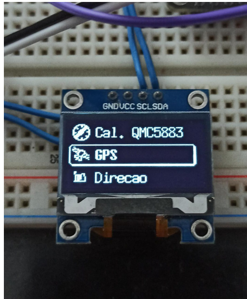
Figura 7 – Display OLED 128x64.
