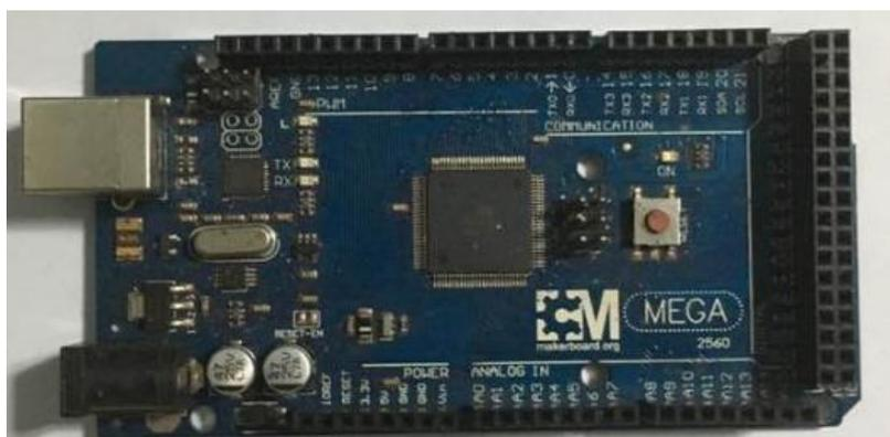
**Figura 7 – Placa Arduino MEGA 2560.**
