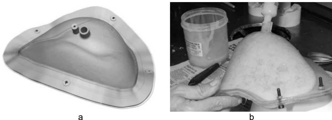
Caption: a. custom breast mold b. the cast, closed, receiving manual silicone rubber injection
