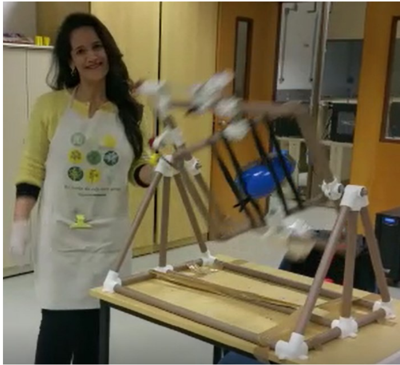
Figure F 3 – The "rotomolding" machine, in operation
