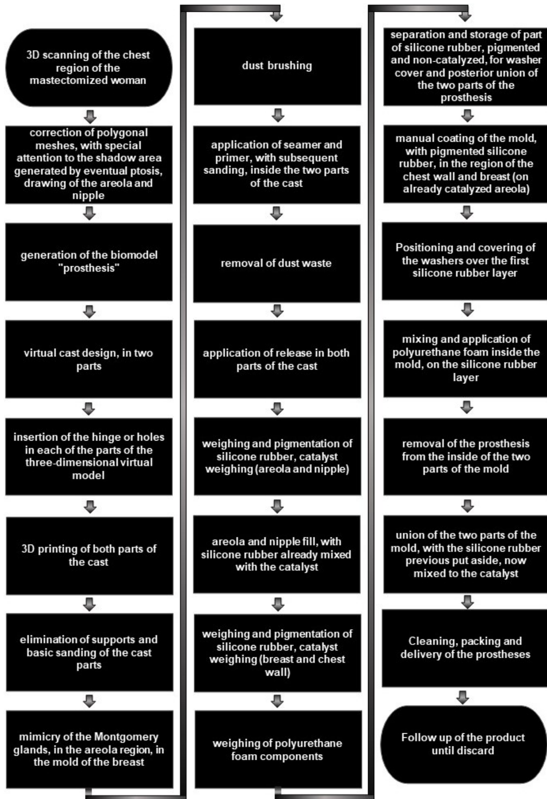
Figure 53 – Flow chart for manufacturing personalized external breast prostheses
