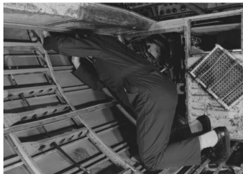
Figure 1.2 – Difficult access Source: Moscheto (2009)
