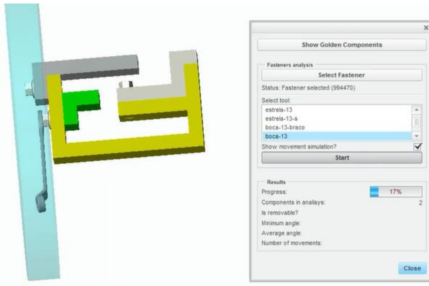
Figure 4.51 – Illustrative example – Interference volume on F3 removal
