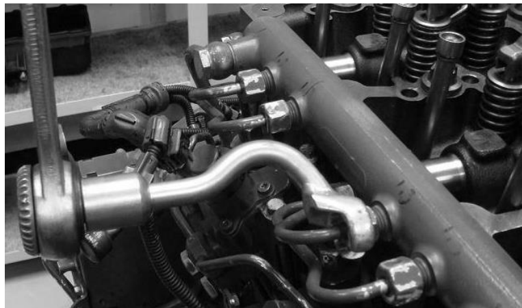
Figure 2.7 – Special tool made from universal tools Source: Adapted from Moscheto (2009).
