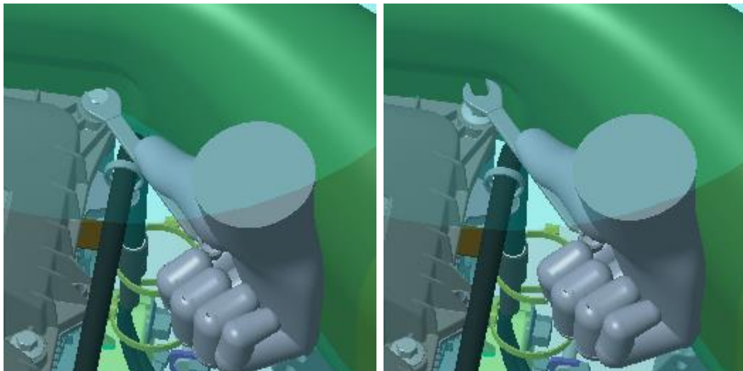
Figure 4.62 – Valve cover access analysis with regular wrench – two positions
