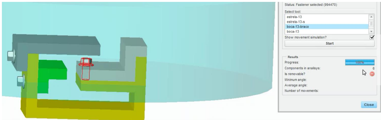
Figure 4.39 – Illustrative example – not possible to remove with P95 hand
