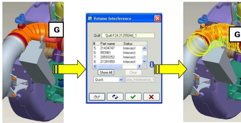
Figure 2.44 – Interference analysis in space claim for maintainability – engine case study Source: Moscheto (2009).
