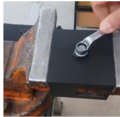
b/ Breaking the fastener torque
