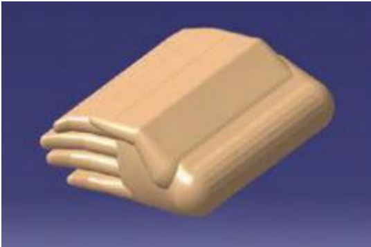
Figure 2.21 – Swept volume to verify maintenance space – Hand volume Source: Zhou et al. (2014).
