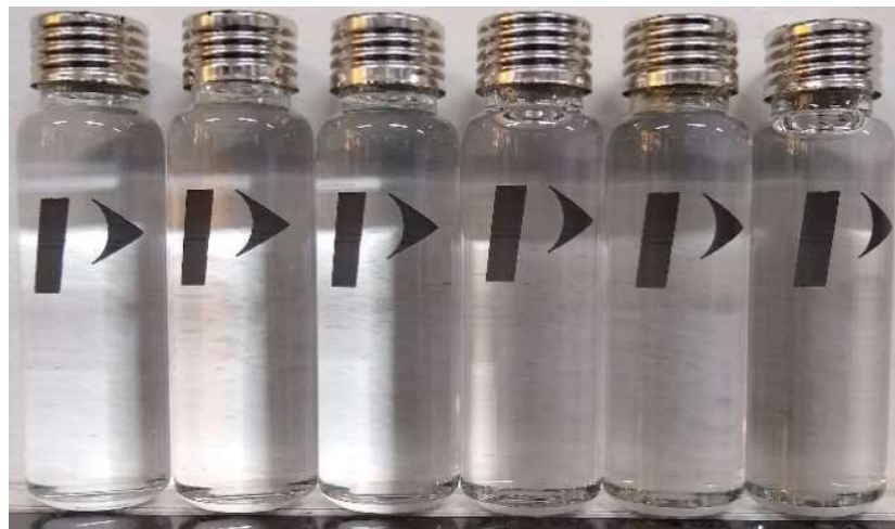
Figure 32 – Glass flasks with pure MEG (from 0% to 100% of MEG)
