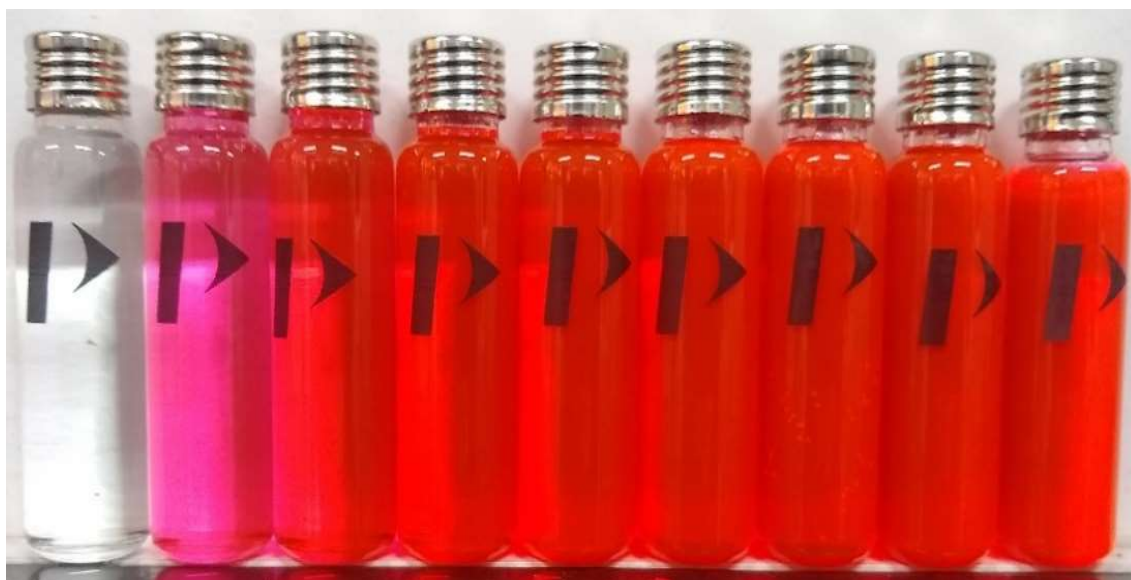
Figure 30 – Glass flasks with dyed MEG
