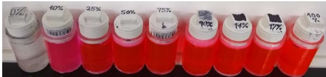
Figure 31 – Acrylic flasks with dyed MEG
