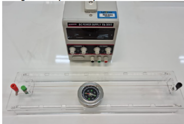
Figura 1 - Aparato experimental de Oersted
