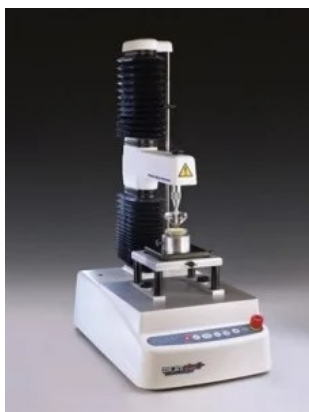
Figura 8 - Texturômetro, modelo TA.XTplus/50, marca Stable Micro System
