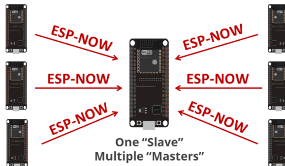
Figura 22 – Multiple master Communication
