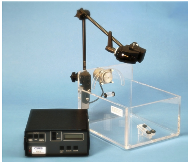
Figura 45 - CIRS Doppler String Phantom model 043.
