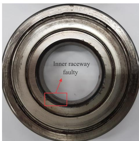
Fig. 8. Faulty bearing removed from the IM after 6 months of operation showing crack in the inner raceway.
