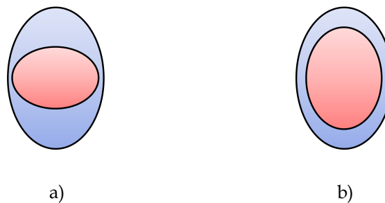
Figure 2-5. Configurations of the compound drop: (a) out-of-phase oscillations; and (b) in-phase oscillations.
