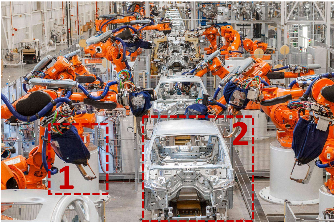
Figure 1.1: Example of a robotic welding assembly line. A robot holding a spot welding tool (1) and a vehicle's body (2) are illustrated.
