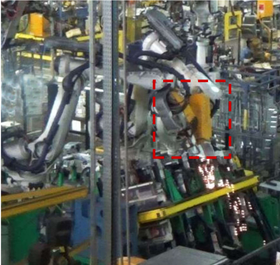
Figure 3.2: Platform robots performing welding tasks at the same time on the same work-piece. The yellow welding guns that each robot holds are highlighted in the picture.
