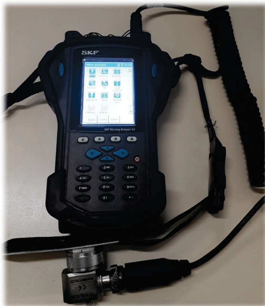
Figura 3 – Aparelho SKF Microlog Analyzer GX CMVA75
