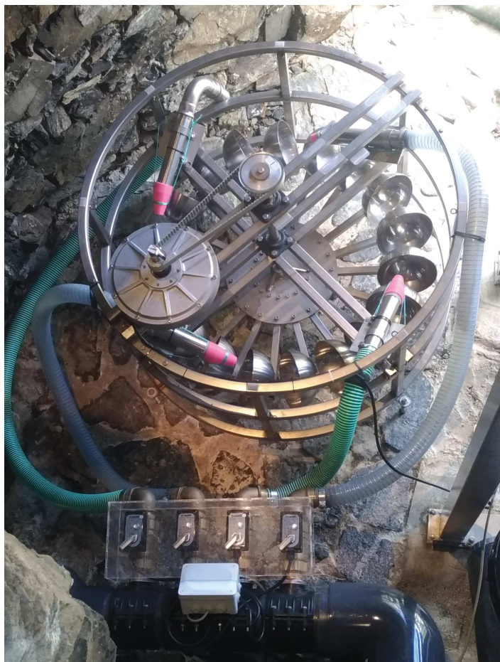
Figure 3.2: Water wheel at House of Silk.
