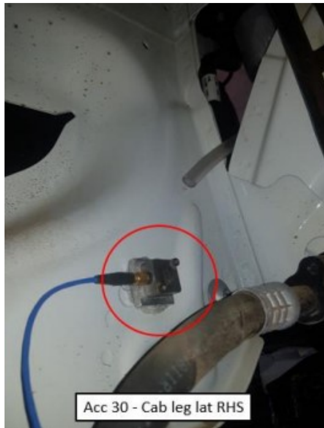
Figure 42 – Example of accelerometer positioning presented within a test report
