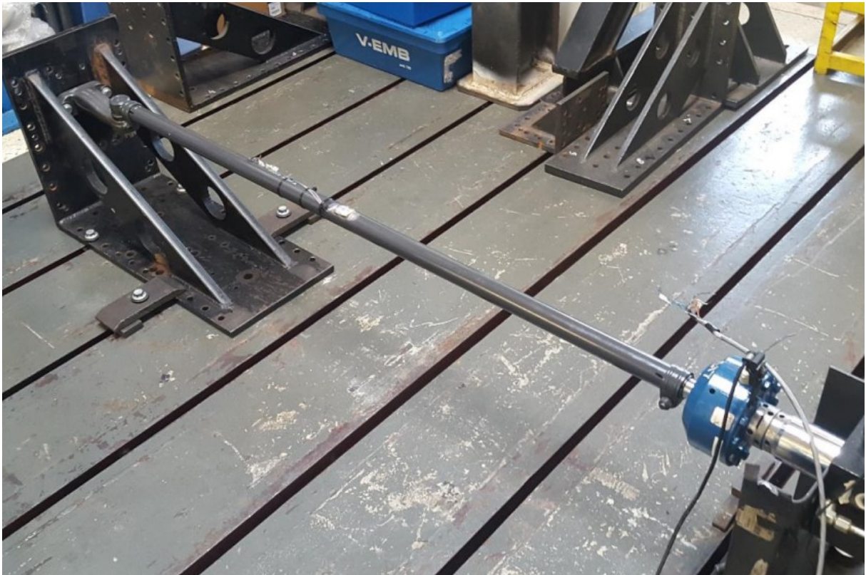
Figure 46 – Steering link calibration for axial forces in a test bench
