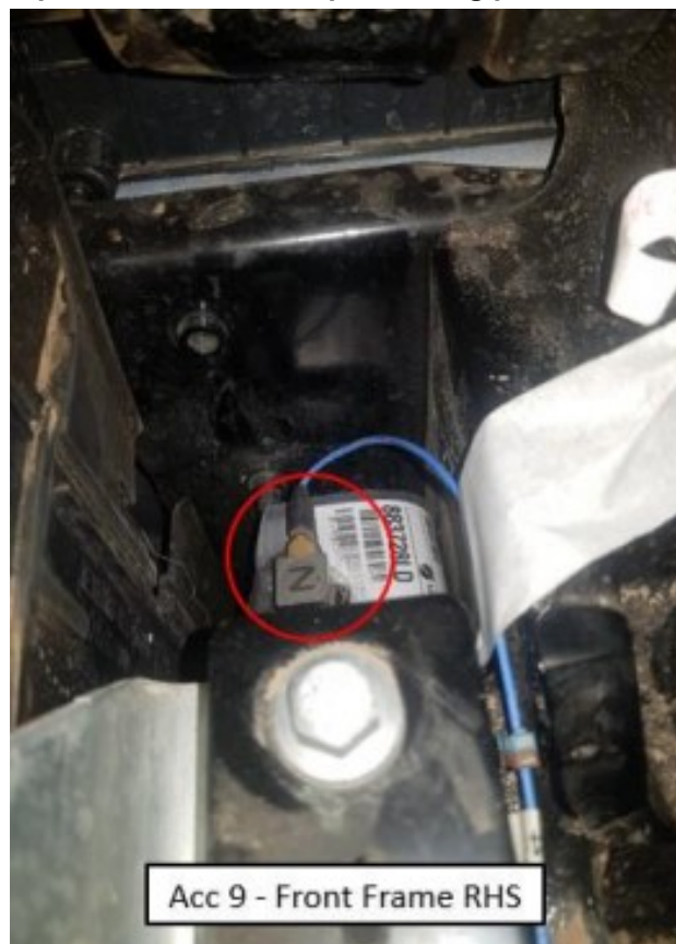
Figure 41 – Example of accelerometer positioning presented within a test report
