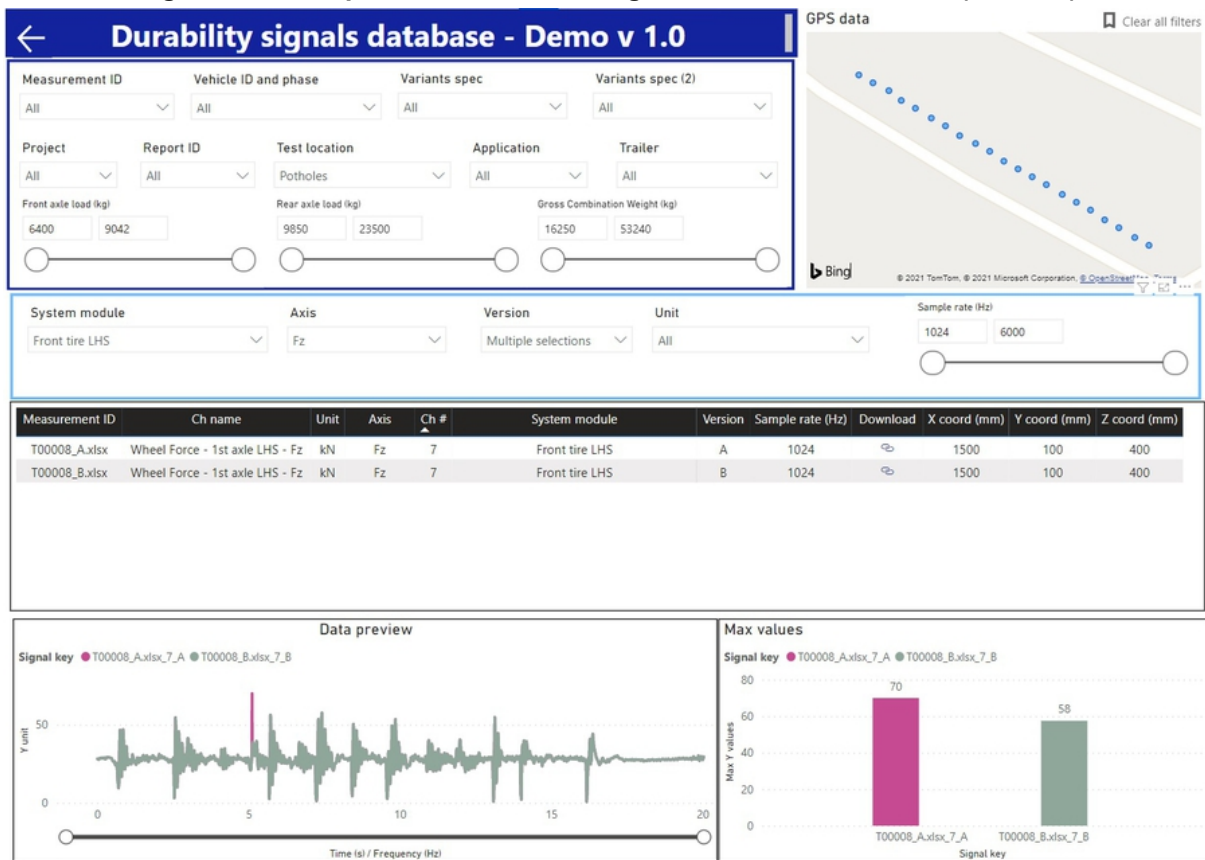
Figure 68 – Comparison of the same signal on different versions (A and B)
