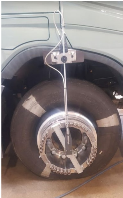
Figure 3 – Wheel force transducer installed in a commercial vehicle
