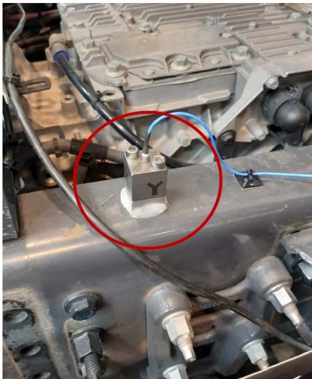
Figure 5 – Triaxial accelerometer installed in the frame of a commercial vehicle
