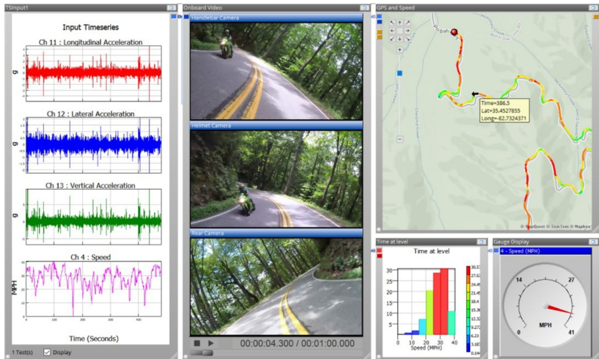
Figure 38 – Time-synced GPS and channel data example
