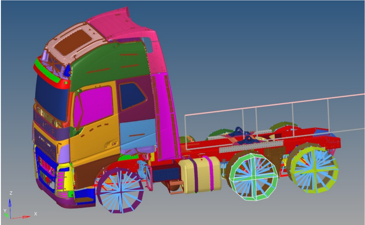
Figure 54 – Complete vehicle model generated based on the product structure data for PROTO_23:01_T
