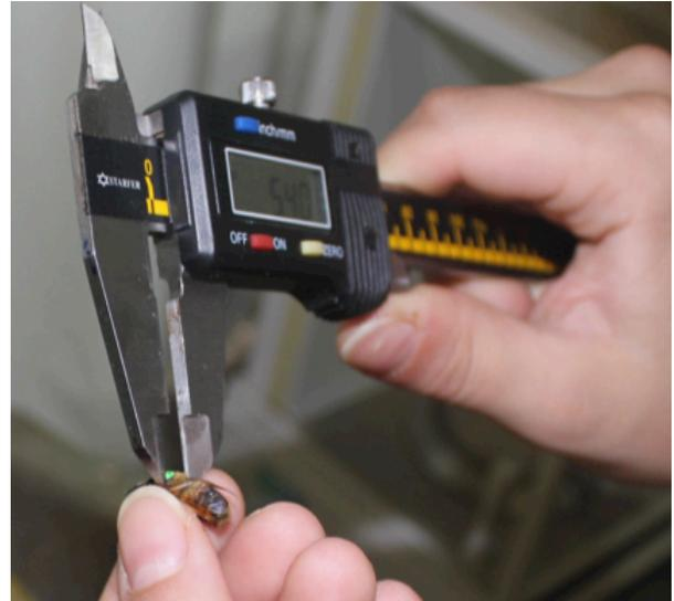
**Figure 3 and 4. Drone weighing in a analytical scale, Shimadzu/AX 200. Measuring abdomen length with a digital caliper (Starfer-150 mm, with a maximum resolution of 0.01 mm), respectively. Source: Rodrigues (2013)**
