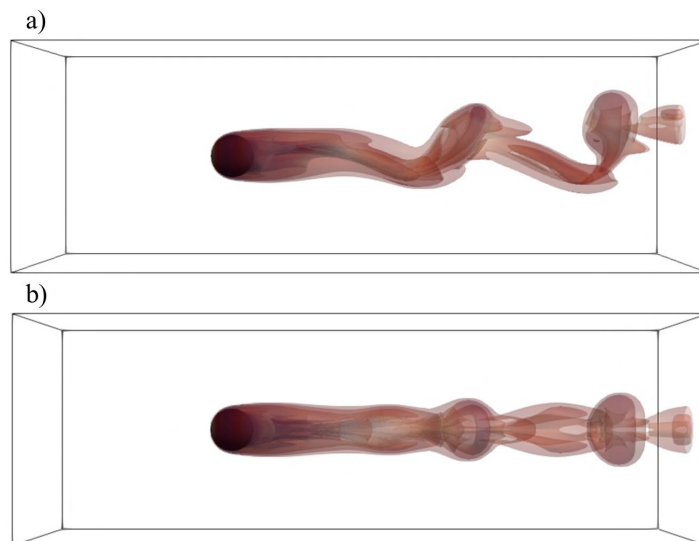
Figure 30 – Vorticity surfaces for Re = 420 , (a) side view and (b) top view.
