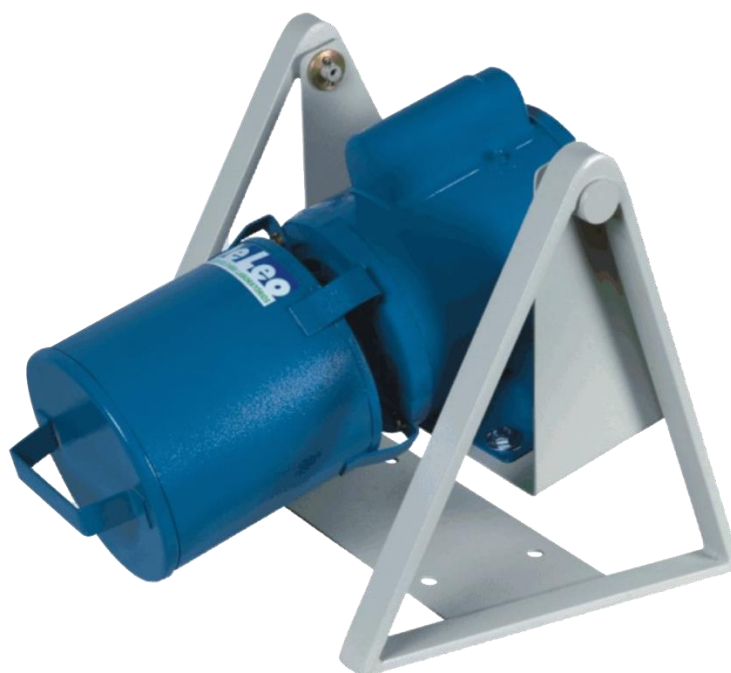
Figure 55. Rotational scarification machine (De Leo®) used to scarify husked seeds. The electric motor on the right turns on the chamber on the left which is lined with sandpaper. Seeds are placed inside the chamber and the handle allows to swing the system and promote homogeneity. Level of scarification can be controlled by the time of the process ( Picture source: De Leo® laboratory equipments ).
