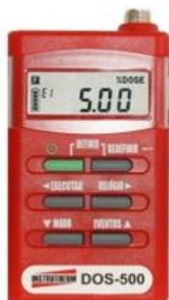
Figura 07: Dosimetro (Instrutherm, LCD, RS232, mod. DOS 500)
