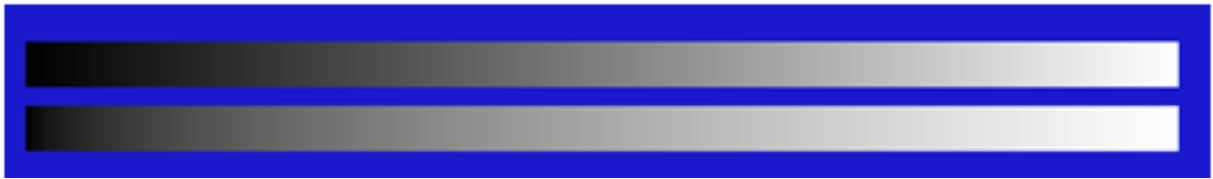
Figure 17: Effect of Gamma correction on the encoding of grayscale values. Upper encoding is the original one. Lower bar represents the encoding after gamma correction.
