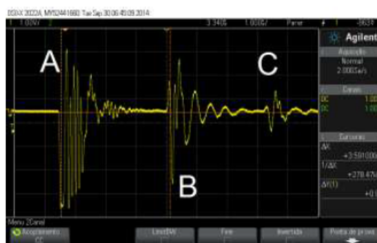
Figure 1: Typical pulse-echo experimental waveforms. Pulse-echo waveform from the top coat. (a) Initial pulse echo transducer, (b) First pulse-echo from the end of IN 718 substrate, (c) Second pulse-echo from the end of sample
