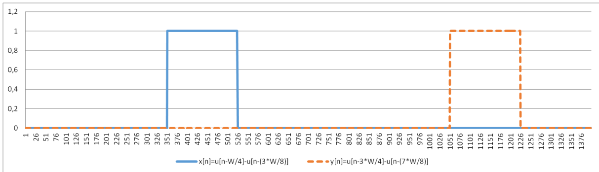
(a) Pulso x(n) = (u(n - W/4) - u(n - (3 * W/8))) e y(n) = u(n - 3 * W/4) - u(n - (7 * W/8)) , com W = 1400 .
