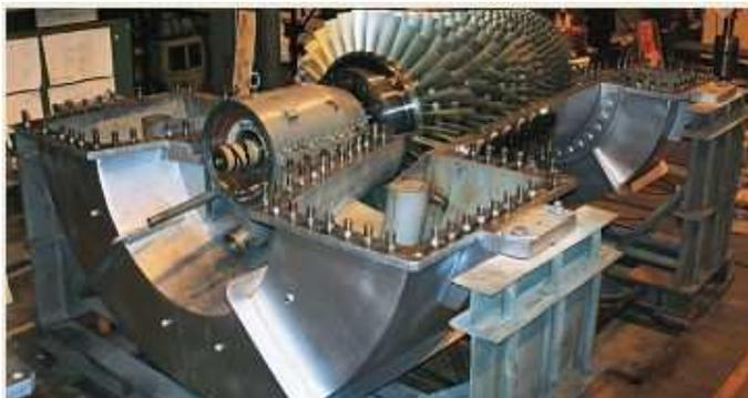
Figura 03 – Compressor Axial
