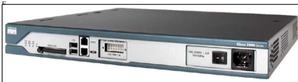
Figura 7. Roteador Cisco Integrated Services Modelo 2811.
